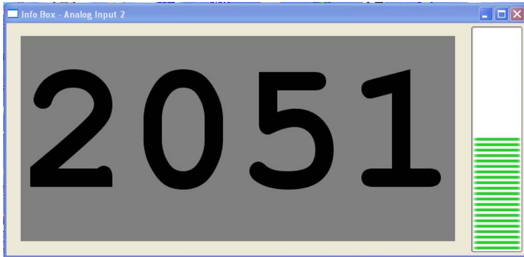
Large "billboard" display of selected input channel. Display includes numeric value (0 to 4096) and bar graph on the side.
